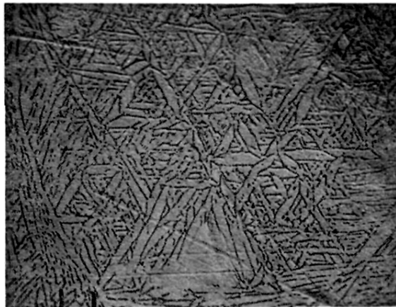
FIG. 5. Optical micrograph of Ti-1 Mn after first quenching from 1000°C (Fig. 4), then annealing for 8 h at 690°C and quenching to -190°C. Note mesh-like array of \beta phase filaments in \alpha -phase matrix. Fiducial marks indicate 10 \mu .
