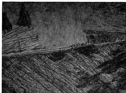
Fig. 6. Optical micrograph of as-cast (argon arc melted) Ti-1 Mn. This is probably a mixture of \alpha , \alpha' , and \beta phases. See Refs. 30 and 31. Note grain boundary of parent \beta phase. Fiducial marks indicate 10 \mu .
