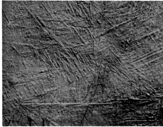
FIG. 4. Optical micrograph of Ti-2 Mn annealed at 1000°C and quenched rapidly ( \approx 0.6 sec) to -190^{\circ}\text{C} . This structure is characteristic of the \alpha' martensite phase. Fiducial marks indicate 10\ \mu .
